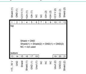
Terminal assignment for mounting rail version, 3 or 4 channel
