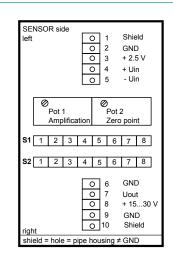
Terminal assignment for mounting rail version, 2 channel
